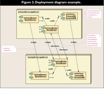
found in implementation model diagrams, such as component diagrams and deployment diagrams. A component diagram shows the organization and dependencies of components, and a deployment diagram shows how component and class instances are deployed on computational nodes. An example of a deployment diagram that uses components is shown in Figure 2.
